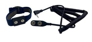
Dual wire wrist straps are designed to work with dual wire resistance style, constant monitors. The wrist band is fully adjustable that stay flat on the wrist for good contact. Which provides redundancy – even if one dual wire wrist strap conductor is served, operator has reliable path-to-ground with other wire.
